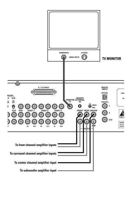
**Figure 4: Input Connections**
